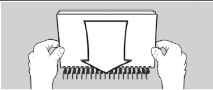
**3D** Assemble pages onto open comb. Remove the sheets from the punch slot and insert onto the fingers of the binding comb.
