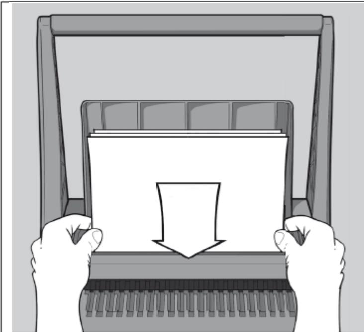
**3B** Load pages into slot. You can punch 2 cover sheets or up to 20 sheets of paper (20lb./80gsm) at a time.
