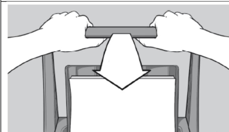
**3C** Punch pages by pulling handle down. Then lift the handle back to the vertical position and remove the punched sheets. Note: To prevent jams do not attempt to punch more than two cover sheets at a time.
