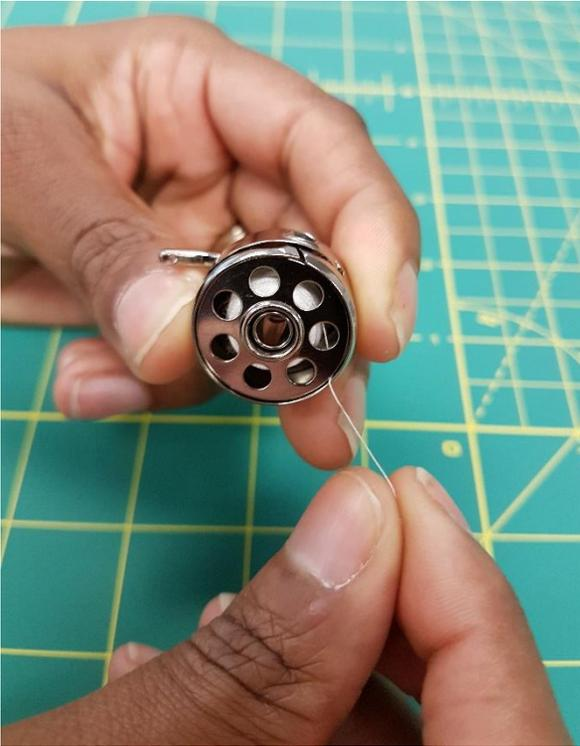
Take the thread anticlockwise to the slot
