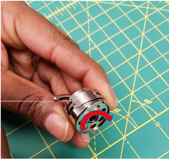
When the end of the thread is pulled, the bobbin should turn clockwise, in the direction of the arrow.
