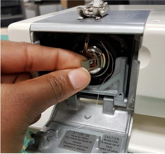
Hold the bobbin case by the latch with the index finger and thumb of the left hand. Insert so that the finger of the bobbin case points upwards, engaging in the notch of the hook race cover.
