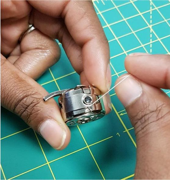
Pull the thread into the slot and under the spring, until it lies in the T-shaped slot at the end of the spring.
