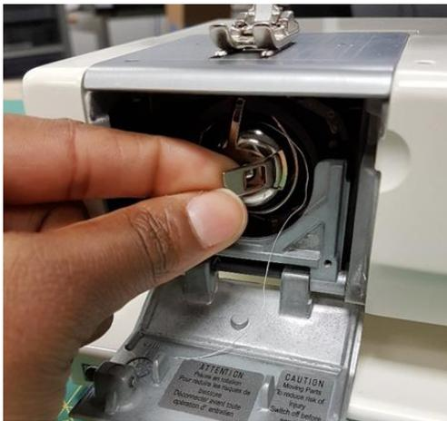
Hold the bobbin case by the latch with the index finger and thumb of the left hand.
