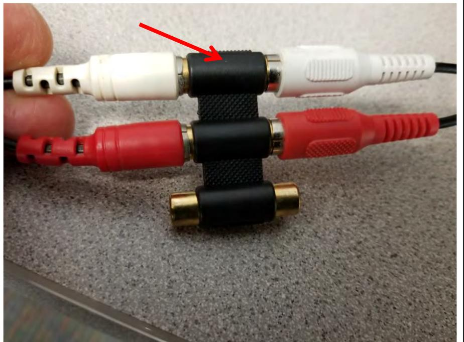
Now connect the audio cable to the Roxio USB capture device, once again being mindful of matching the white cable into the white input slot on the Roxio adapter. Do the same for the red cable by inserting into the red input slot.
