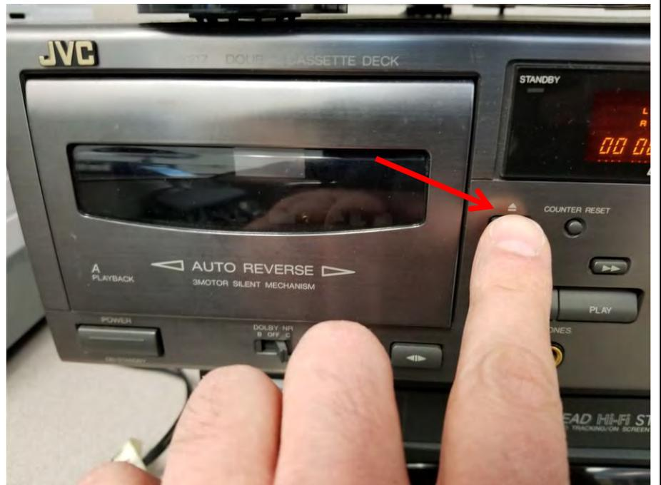
Load up an audio cassette, ensuring that the tape side is on the bottom when inserting the cassette into the cassette deck. Side A of the cassette should be facing you.
