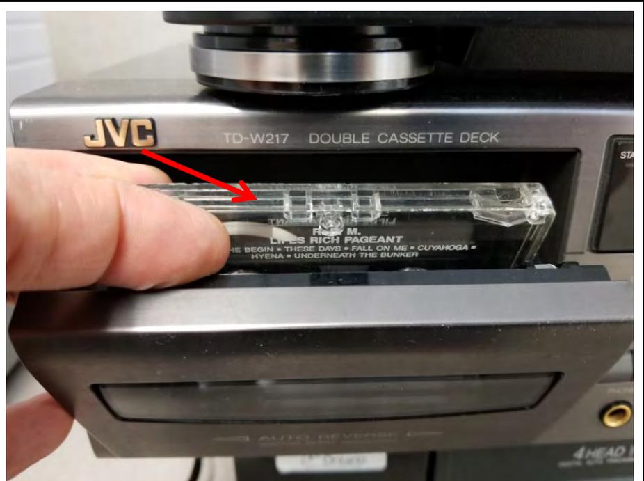
Close the door on the cassette deck. Couple of things to note here. The first thing you should do is rewind the tape marked by **two left facing triangles**. Once the tape is rewound, you can press **COUNTER RESET** to put the counter back at 00:00 time code. Lastly, ensure that the **REVERSE MODE** switch is set to the middle for one automatic palyback of the reserve side of the tape. This will ensure that you don't need to flip the cassette once Side A has finished.
