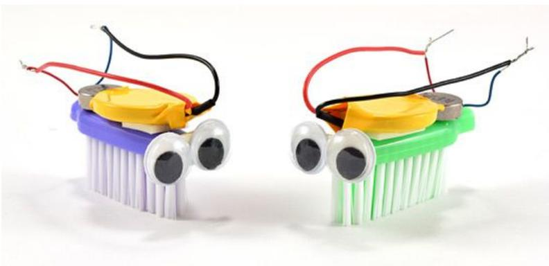
If you want to add motors to your robot, maybe you can find an old toy or device that can be scrapped for parts. Even a small motor can be used to make simple robots that move. Check out the "bristlebot", a robot that races around the floor using just a brush head, coin cell battery, and a small vibration motor.
